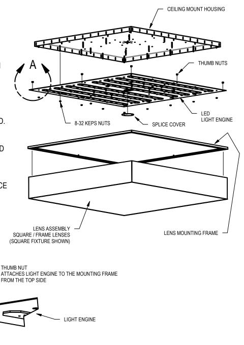
KEP NUTS ATTACHES THE LIGHT ENGINE TO THE CEILING MOUNT HOUSING FROM THE BOTTOM SIDE
