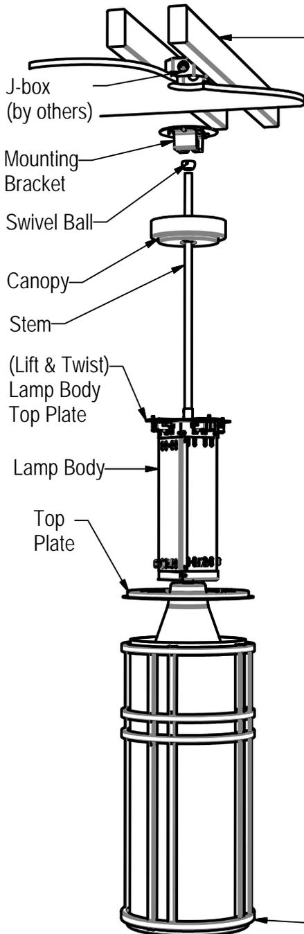
Auxiliary Structural Mounting - Because fixture weight may exceed the structural capacity of a standard electrical box, additional structural mounting is required (by others.) **Note:** Mounting bracket has two mounting slots for auxiliary support.
