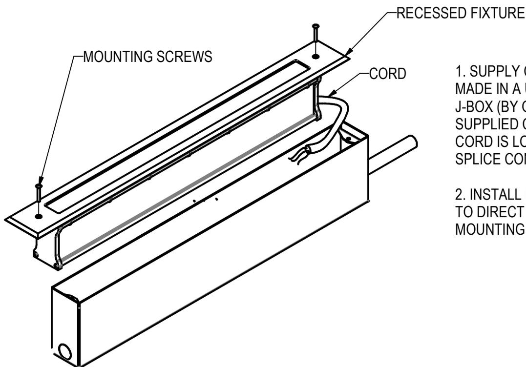
1. SUPPLY CONNECTIONS TO BE MADE IN A UL LISTED LIQUID TIGHT J-BOX (BY OTHERS). WHEN CUTTING SUPPLIED CORD, ENSURE THAT THE CORD IS LONG ENOUGH TO REACH SPLICE CONNECTION.
