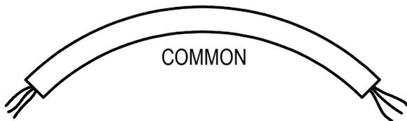
COMMON SEGMENTS HAVE CONNECTION WIRING AT BOTH ENDS.
