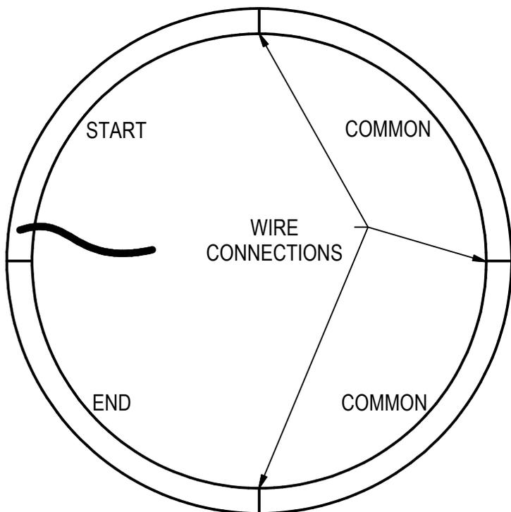
MAKE WIRE CONNECTIONS BETWEEN SEGMENTS AS SHOWN IN THE EXAMPLE DIAGRAM. THERE WILL BE NO CONNECTION MADE BETWEEN THE START AND END SEGMENTS OF A RING.
