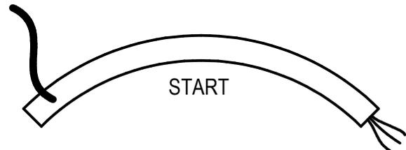
START SEGMENTS HAVE A POWER CORD ON ONE END, AND CONNECTION WIRING AT THE OPPOSITE END.
