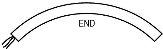
END SEGMENTS HAVE CONNECTION WIRING AT ONLY ONE END.
