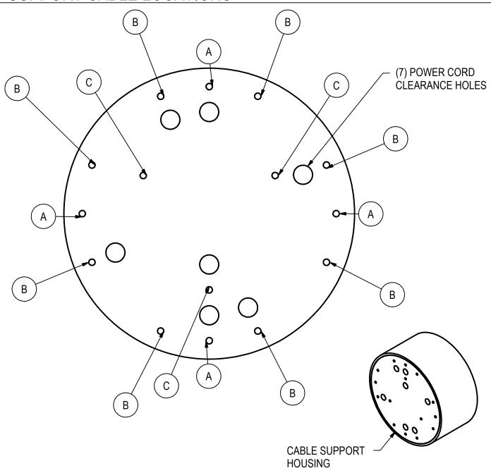
"A" = (4) AIRCRAFT CABLE MOUNTING FOR 72" DIAMETER RING FIXTURE.
