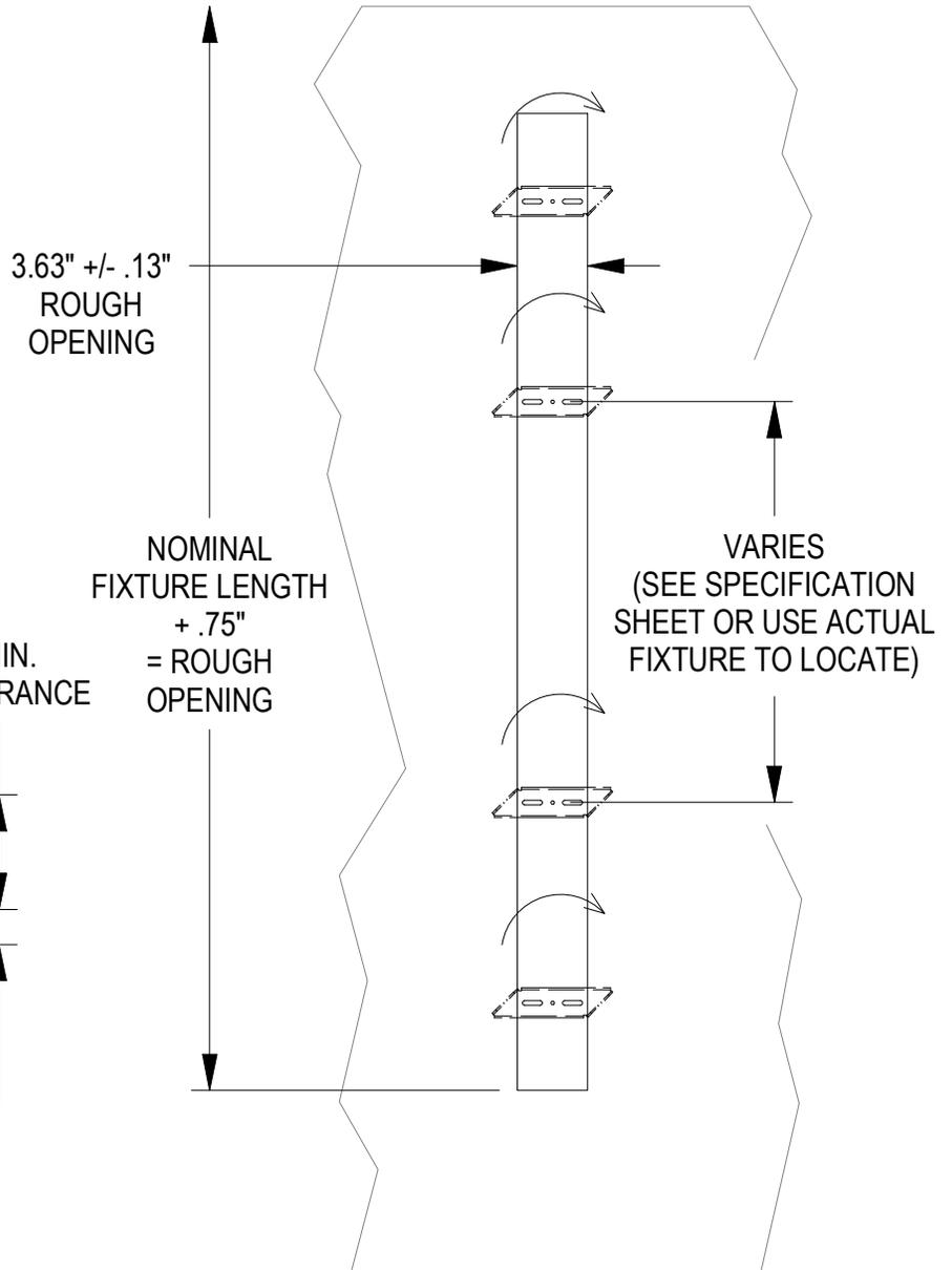
**A** SURFACE SUPPORTING WITH PIVOT MOUNTING BRACKET
