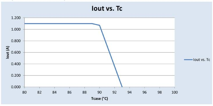
Note: There is ±5°C tolerance on the driver case temperature.
